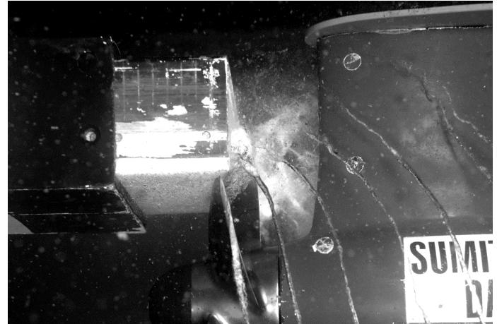
Figure 2: Cavitation extent as an ice block impacts a propeller
