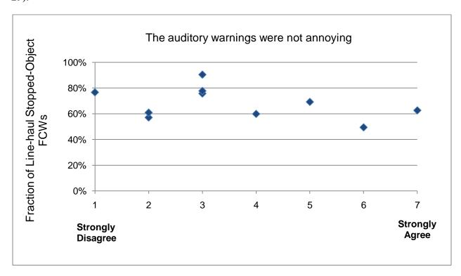
Figure 29: Fraction of "stopped object" Forward collision warnings versus line-haul drivers' responses to Q18.
