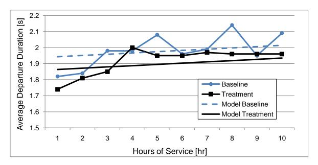
Figure 59: Lane departure duration for both experimental conditions versus hours of service for the steady-state left lane departure events on limited access.
