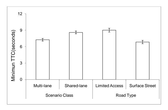
Figure 114: Effects of scenario class and road type on minimum time to collision
