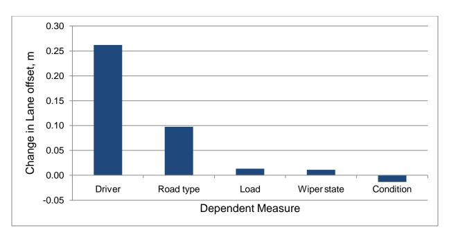
Figure 77: Relative change in lateral offset as function of driver and other dependent measures.
