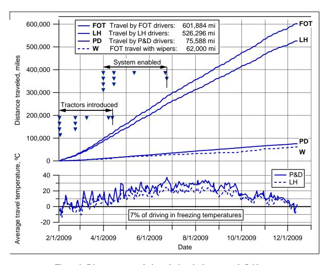
Figure 9: Distance accumulations during the heavy-truck field test
