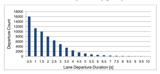
Figure 65: Histogram of lane departure duration during steady-state lane keeping events.
