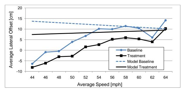
Figure 44: Average lateral offset for both experimental conditions versus the average speed during steady-state lane keeping for travel on limited access roads.
