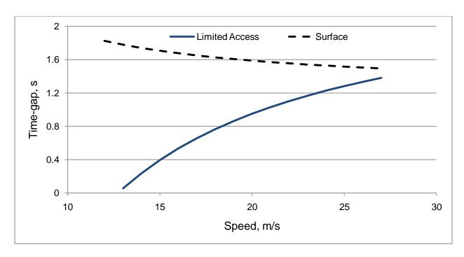
Figure 92: POV2 time-gap as a function of speed for both road types
