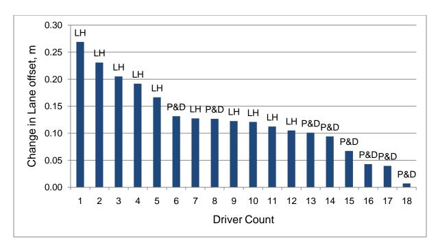
Figure 76: Change in lateral offset caused by an occupied vs. unoccupied adjacent lane on the left for each driver
