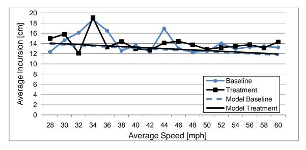
Figure 64: Average maximum incursion for both experimental conditions versus speed for the steady-state left lane departure events.
