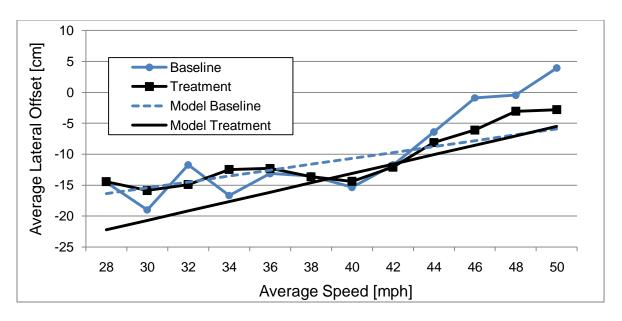
Figure 43: Average lateral offset for both experimental conditions versus the average speed during steady-state lane keeping for travel on surface streets.
