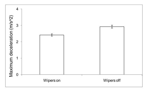
Figure 119: Least squares means of maximum deceleration with different wiper states
