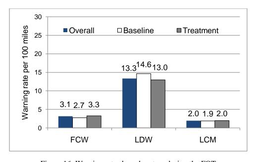
Figure 16: Warning rates by subsystem during the FOT
