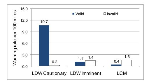
Figure 39: Overall lateral warning rate per 100 miles for each warning type.
