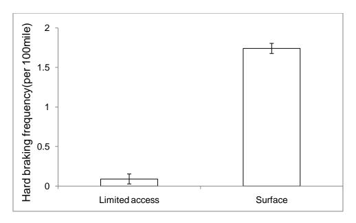
Figure 117: Least squares means of hard braking frequency on different road types
