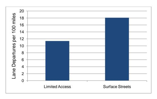
Figure 51: Least square means of lane departure rates for road type during steady-state lane keeping.
