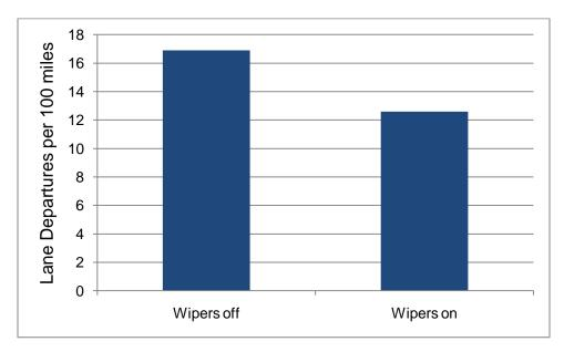
Figure 52: Least square means of lane departure rates for wiper state during steady-state lane keeping.
