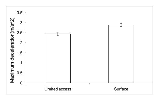
Figure 118: Least squares means of maximum deceleration on different road types
