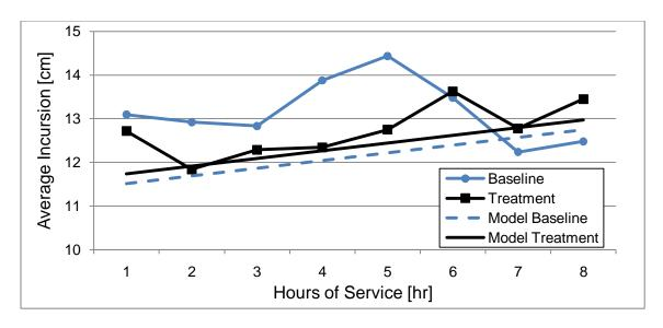
Figure 63: Average maximum incursion for both experimental conditions versus hours of service for the steady-state left lane departure events.
