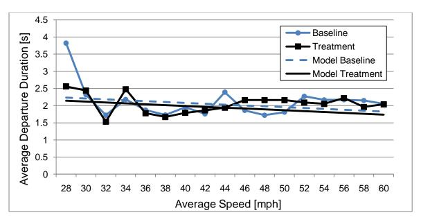
Figure 60: Lane departure duration for both experimental conditions versus speed for the steadystate left lane departure events on limited access roads.
