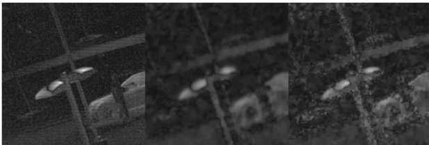
Fig. 7. Estimates of the DOLP for SNR=15 dB; from left to right: pristine, proposed method with cross-channel regularization, traditional method with cross-channel regularization.
