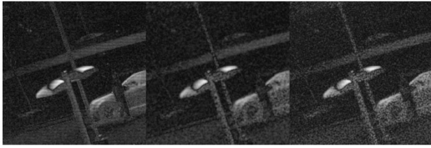
Fig. 4. Estimates of the DOLP for SNR=25 dB; from left to right: pristine, proposed method, traditional method.
