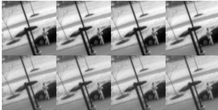
Fig. 1. Noisy and blurred polarimetric imagery. The first row has an SNR of 25 dB and the second row has an SNR of 15 dB. From left to right the angle of the polarizer is \{0^\circ, 45^\circ, 90^\circ, 135^\circ\} .
