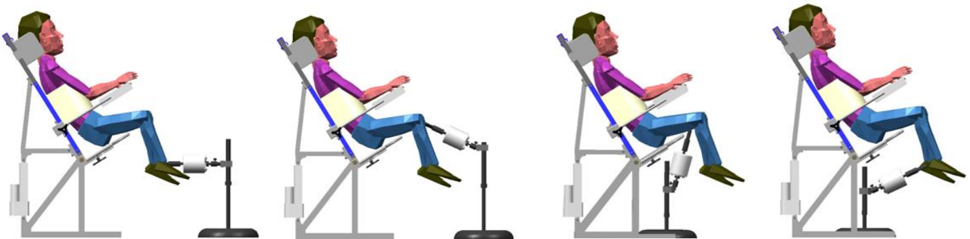
Figure 28: Ball joint's full range of motion is used to properly place the pulsator at each testing site.
