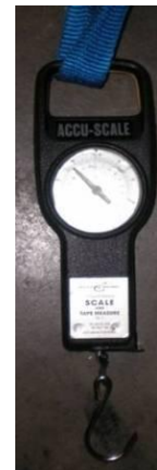
Figure 35: Force gauge with resolution 0.5 lb
