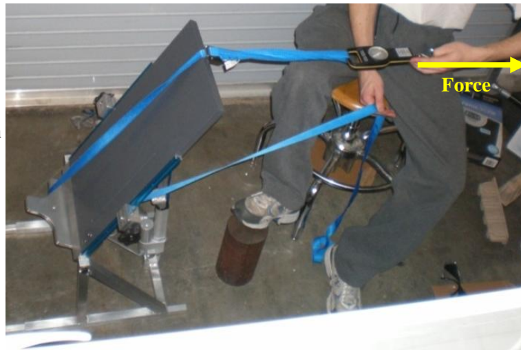
Figure 36: Force applied on top rope by pulling on force gauge causing the chair to tip (backwards tipping)
