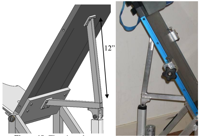
Figure 18: The triangular mount connects the linear actuator to the PVC back rest and the aluminum rotator piece. CAD model on left, prototype on right.
