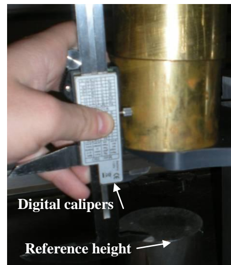
Figure 34: Measuring deflection of seat pan tip against reference height
