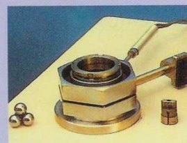
4-Ball E.P.wear cup, chuck, welded balls
