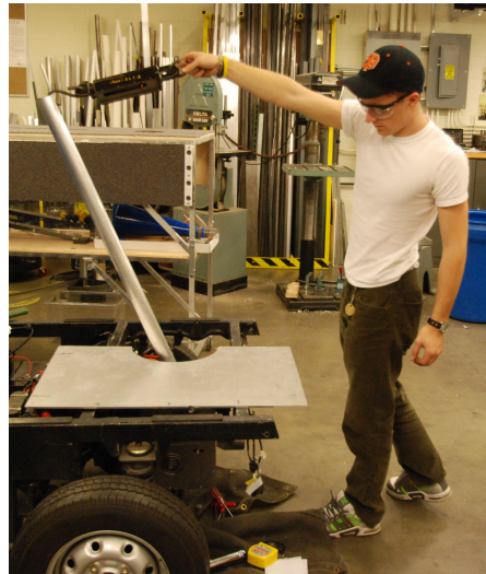
Figure 7.1: Applying torque to reduction housing
