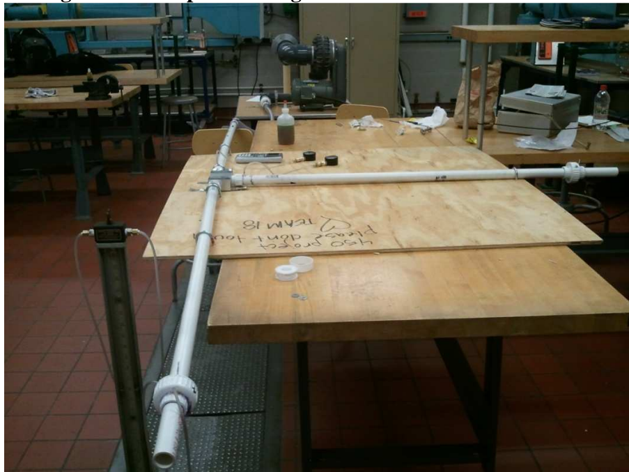
Figure 27: Complete test rig with valve and blower attached
