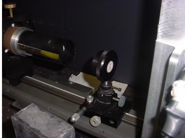
Figure 5-34. Na-22 source disk (60uCi) in the cylindrical holder.
