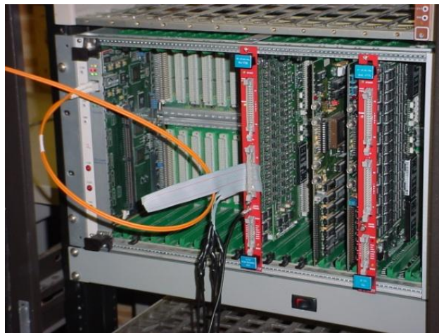
Figure 5-11. VME (Versa Module European) interface card (far left) and a V785 peak-sensing ADC card (the second one from the left).
