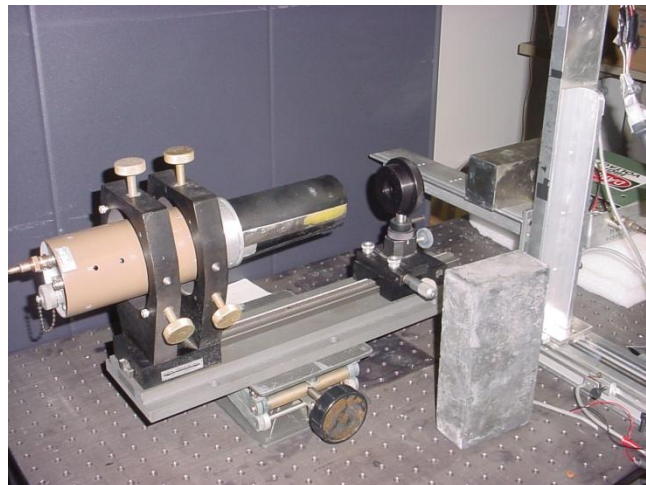
Figure 5-35. Coincidence set-up for the gain adjustment.
