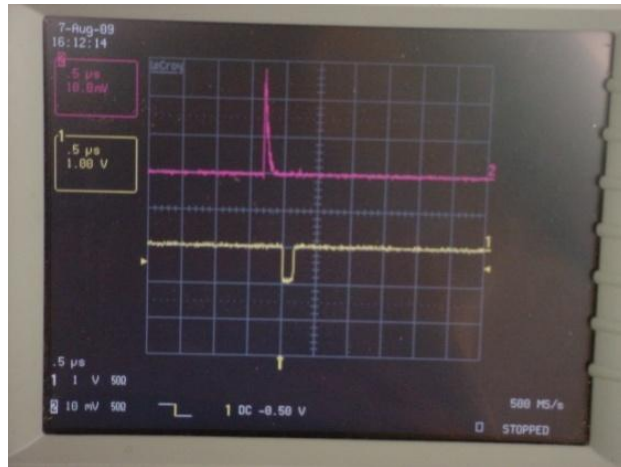
Figure 5-32. LSO dynode signal and the trigger signal from a constant fraction discriminator. The trigger pulse is about 250 ns behind the dynode signal.
