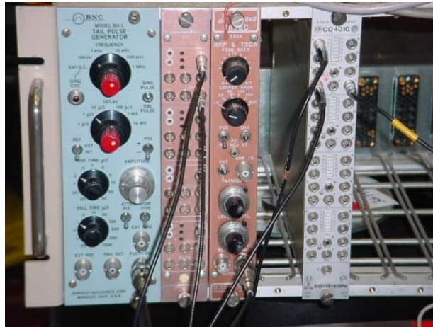
Figure 5-8. Tail pulse generator (far left). The tail pulse generator produces exponentially decaying pulses. These pulses power the LED that simulates scintillation pulses.
