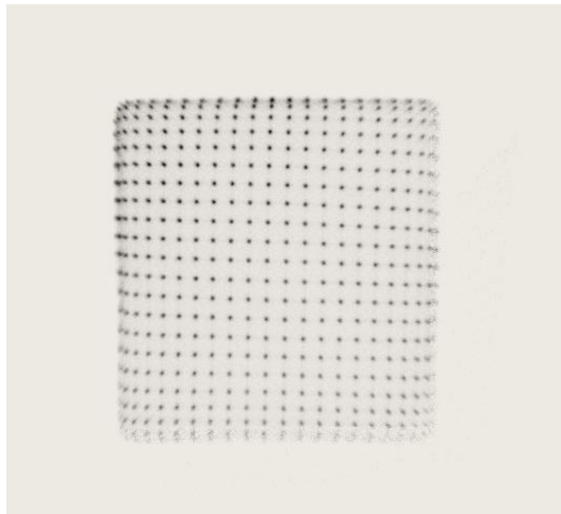
Figure 5-59. Flood image of Na-22 in NaI(Tl) at -750V. The image size is a 512-by-512 array of pixels.
