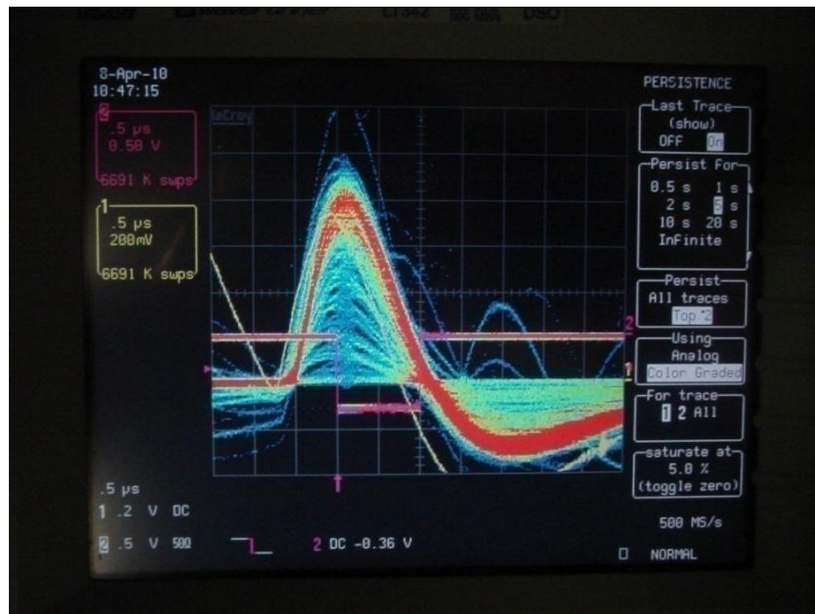
Figure 5-43. Coincidence gate pulses and shaped BGO signals from one channel.
