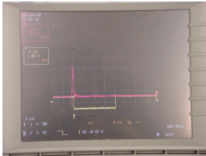
Figure 5-10. Sum signal of 4 outputs from the CDC circuit (the positive analog signal). The gate pulse for the peak-sensing ADC (the negative pulse).
