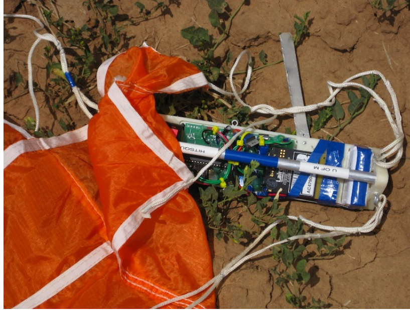
Figure 5.1 Cansat payload shown as found post-flight, with the parachute attached (Hitsquad Team, 2009).
