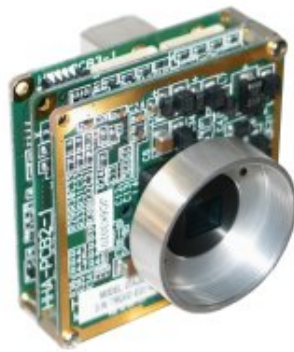
Figure 6.5 Sentech C202 USB CCD camera (Sentech America, 2006).
