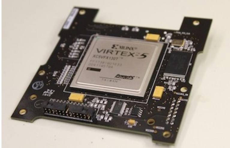
Figure 6.27 M-Cubed's secondary payload, JPL's Xilinx Virtex-5 FPGA that hosts the algorithm to meet MSPI's on-board processing requirements (ESTO, 2010).
