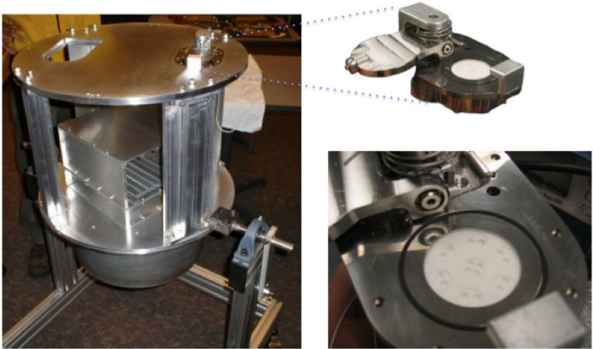
Figure 1.3 The Field Emission Get-Away-Special Investigation proto-flight unit NASA GAS Reservation G-187 (left) with close up of Small Vacuum Protective Enclosure (right) (Ramos & Liu, 2005).
