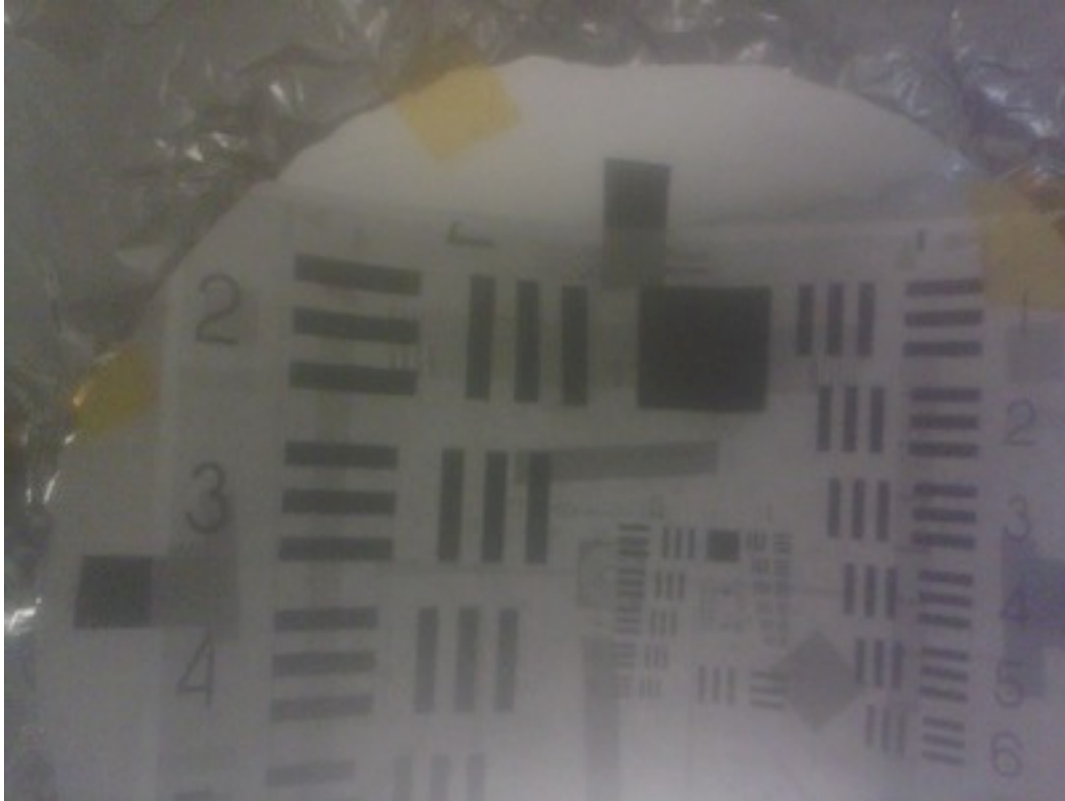
Figure 6.14 M-Cubed primary payload's image captured during vacuum test at 4.03E-05 Torr. The target observed in the image is a resolution chart at 55 cm.
