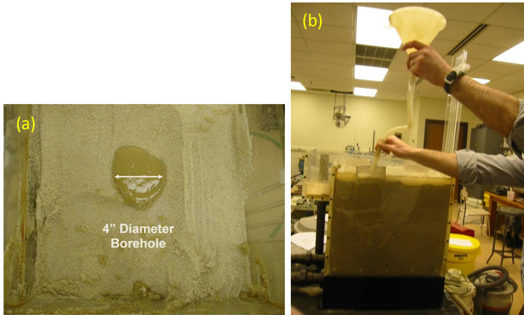
Figure 4-24. Tests performed in a liquefaction tank were used to determine the amount of bentonite in the slurry mix. (a) Slurry maintained a 4" diameter borehole during liquefaction. (b) Poring slurry into the bore hole.
