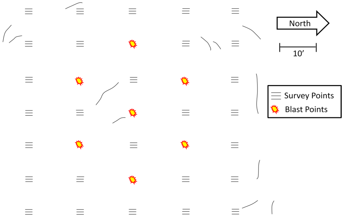
Figure 4-40. Surface cracks observed following explosive densification.
