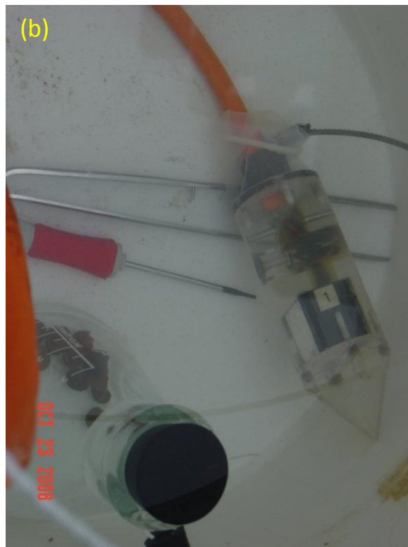
Figure 5-3. (a) Stable PPT and (b) unstable pore pressure transducers and accelerometers in the same cone (photos courtesy of Russell Green).
