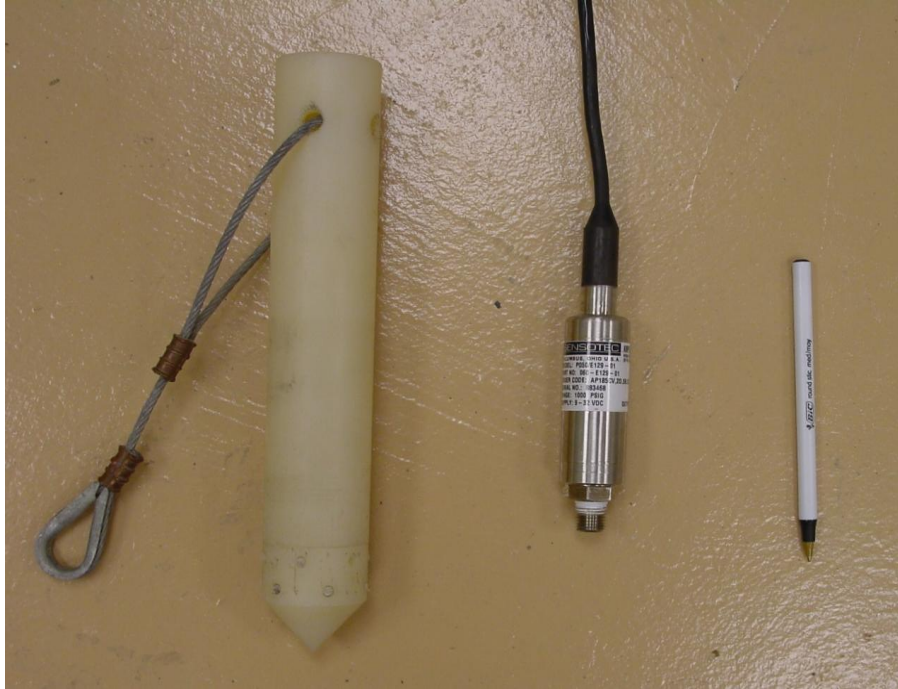
Figure 4-13. Sensotec pore pressure transducer with nylon cone.
