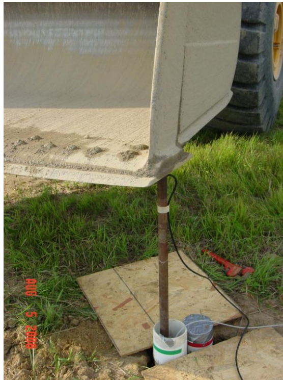
Figure 4-25. A large loader was used to push the instrumentation 1' into undisturbed soil (photo courtesy of Russell Green).
