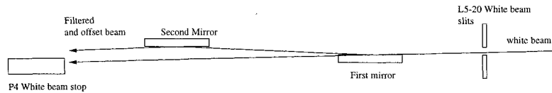
FIGURE 1. The double mirror filter set up.
