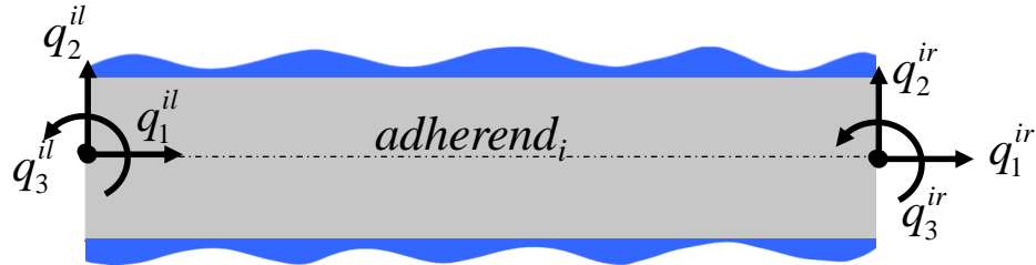
Figure 2-2: Boundary conditions for adherend i : prescribed nodal displacements and rotations at x=0 and x=l .
