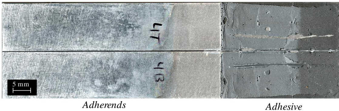
Figure 4-29. Two adherends of an EA 9394 DCB specimen after complete failure. Adhesive found on both adherends indicates that failure occurred within the adhesive layer as desired.
