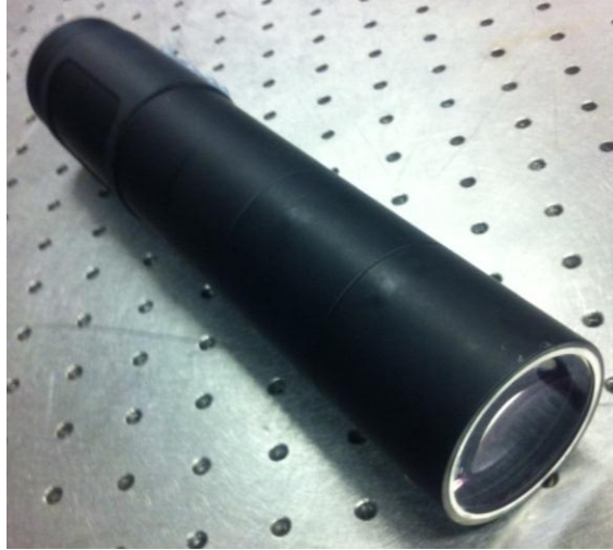
Figure 39: An additional one-to-one imaging optic can be threaded onto the base SC3D-PTV unit to eliminate cross-talk. The additional optic forms an image onto an aperture, and the aperture blocks all light that would cause cross-talk.
