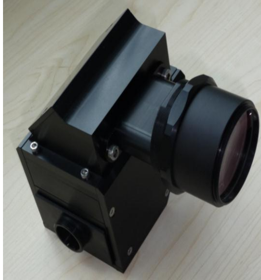
Figure 37: Base unit of the SC3D-PTV imaging system. After the performance of the optical element was simulated, a physical prototype was built. The optics are mounted inside a sealed housing that attaches directly to the camera.
