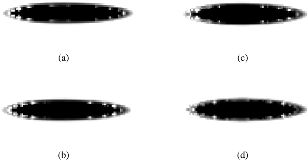
Figure 3.3.15 Design history with the sensitivity filter (a) 19 th step (b) 20 th step (c) 21 st step (d) 22 nd step
