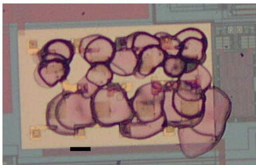
Figure 6.6 Sensor array coated with micro-dispensing system. Top row of sensor are coated with C8 while bottom row is coated with OPH. The scale bar indicates 75 \mu\text{m} .
