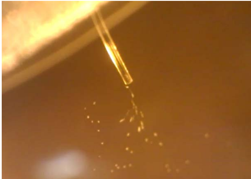
Fig. 3.14 Long-lived micro-bubble generation in the reflected focusing configuration. The fiber hydrophone (125 \mu\text{m} in diameter) was positioned slightly below the water surface which is the reflected focal spot of the LGFU. As soon as the micro-bubbles were generated, they left out of the focal zone.
