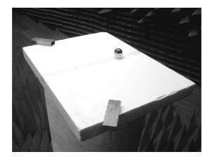
Figure 4.9: Example of anechoic chamber measurements of  $S_{21}$  for a scatterer. The scatterer is a 2 inch diameter conducting sphere. Waveguide apertures in photo are separated by 0.85 m and rotated 40 degrees. The sphere is positioned near the boresights of the waveguide apertures.
