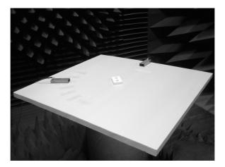
Figure 5.4: Setup for Example 1. The two waveguides are rotated 120 degrees around the target at distances of 16 inches each. The object consists of two acrylic spheres which are separated by approximately 5 cm.
