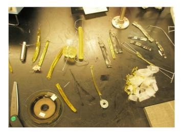
Figure 8.25: Assorted targets of worm rubber, brass rods, and fishline to image.
