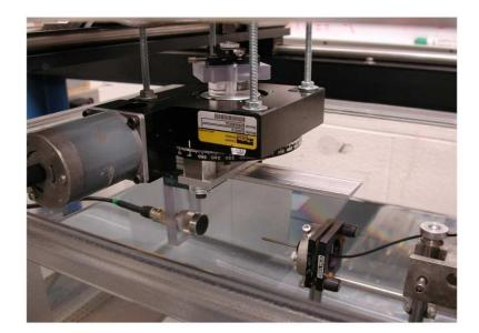
Figure 8.1: Photo of an early hydrophone characterization experiment. A transducer is gimballed and mounted on a translator. The focus of the transducer is positioned at the center of rotation of the rotational stage. A hydrophone is also gimballed and positioned with a 3-axis micropositioner.
