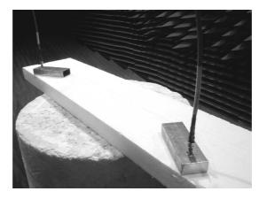
Figure 4.6: Example of anechoic chamber measurements of  $S_{21}$ . Waveguide apertures in photo are separated by 0.55 m and rotated 30 degrees.
