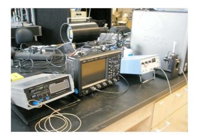
Figure 8.10: Photo of setup to determine the speed of sound of the water bath. From left to right: digital readout thermocouple, oscilloscope, pulser/receiver, micropositioner with transducer and reflection plate.
