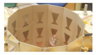
Figure 7.22: Second cavity with antennas designed to operate at 915 MHz of Experiment 2. Three acrylic sphere are suspended (one visible). Cavity is filled with fluid for imaging.
