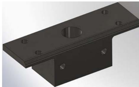
Figure 7: Support Block with Precision Hole for Press Fit.
