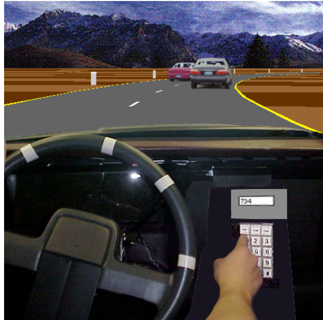
Figure 9. 10-key keypad in the center console location.
