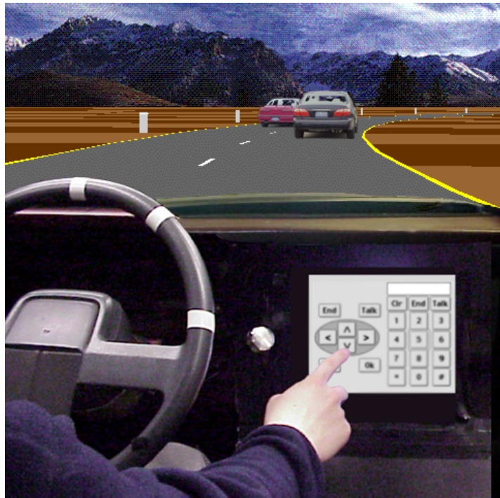
Figure 12. Joystick and its corresponding touch screen display.
