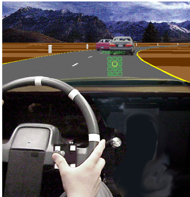
Figure 14. Joystick device on the steering wheel and its HUD display.
