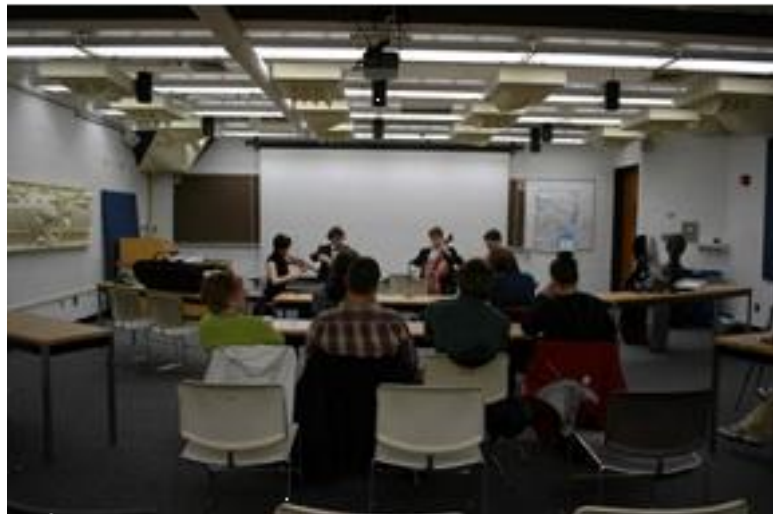
Figure 2.38. An on-site subjective assessment with a string quartet (live music source) and randomly seated respondents. It served as a preliminary research to select the most suitable terms or wording that described the room acoustics conditions.
