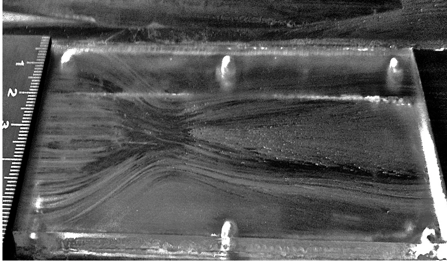
Figure 4.7: Bottom wall oil flow through the UM 3DI-SBLI region. Large corner effects obscure any centerline interaction. Flow from left to right.
