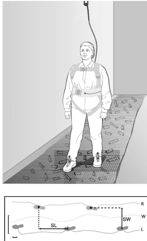
Figure 3-2. Experimental set-up for determining gait speed and step width to step length ratio on an irregular surface. A Figure from Richardson et al. (2005)
