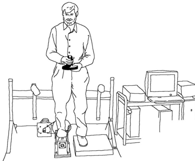
Figure 3-1. Apparatus for determining frontal plane ankle proprioceptive thresholds. Figure from Son et al. (2010).
