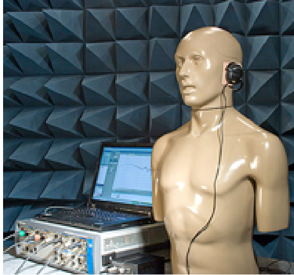
Figure 2.11: Knowles Electronic Manikin For Acoustic Research(KEMAR) used for standardized HRTF measurement
