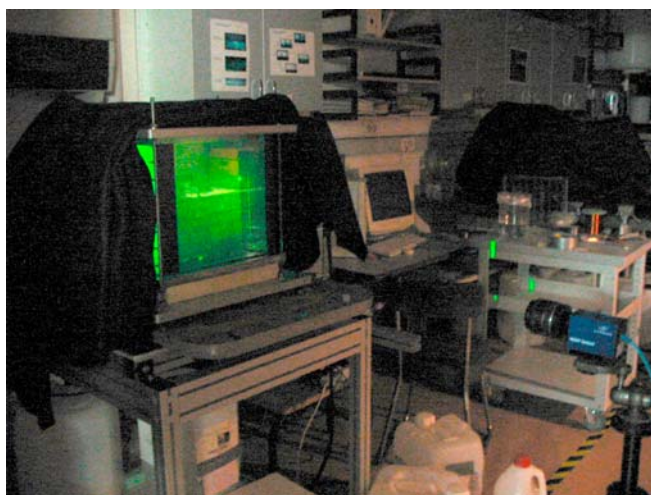
Figure 1. (a) Photo of the laboratory setup (at IPGP) demonstrating the laser sheet (in green), heater assemblage (minor bright point at base of tank), and digital camera. (b) Illustration of the tank geometry and (c) the axisymmetric finite element model. The green area in Figure 1b shows a typical photograph of a plume with temperature contours illuminated by the TLC, and the quadratic elements of the finite element mesh which has a resolution of 0.2 mm near the heater are shown in Figure 1c.
