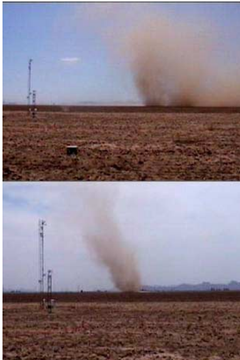
Figure 1. Convective plume and vortex. (top) Large dusty non-rotating convective plume. Plumes are generally 100 m in diameter and persist for nearly an hour. (bottom) Large dust devil. Typical dust devils are generally 10 m in diameter and persist for a few minutes. Both images were taken by N. Renno during the 2002 field campaign near Eloy, Arizona.
