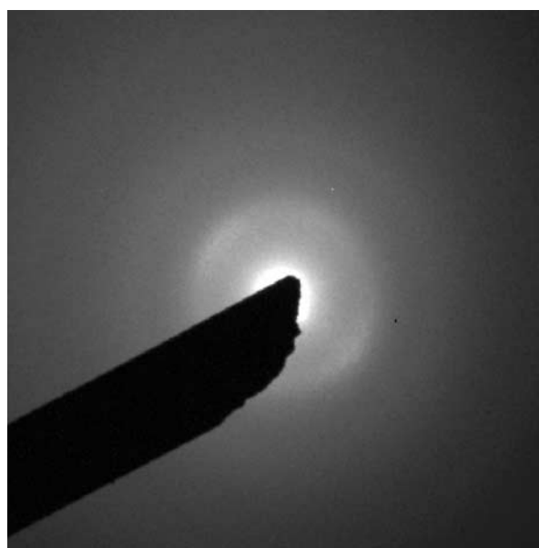
Figure 4. Selected area electron diffraction (SAED) patterns of char particles, indicating an amorphous solid.
