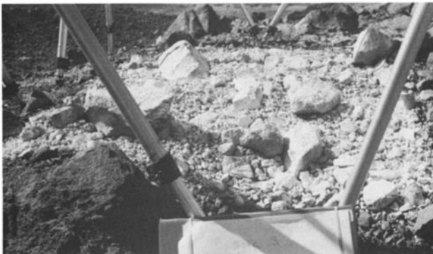
Fig. 3. A sample surface scanned by the EDM. The surface has been spray-painted to increase its reflectivity.
