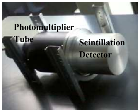
Figure 2– 1: An EJ–309 scintillation detector with its photomultiplier tube.
