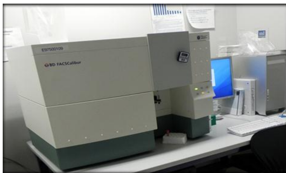
Figure 1.3: Image of a two-laser FACS Calibur Flow Cytometer [adapted from http://www.georgiahealth.edu/cancer/shared/flow/equipment.html ]. The flow cytometer is expensive, bulky, needs electricity and refrigerated reagents and a trained personnel for its operation and maintenance.
