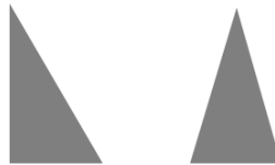
Figure 50: The shape on the left is what was used for the cutting ridges in our prototype because it was easier to manufacture. The shape on the right would be more ideal for the final design because it would eliminate the problem with the cuts not lining up.
