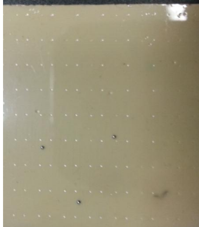
Figure 36: The only beads that stayed in the plastic were the beads that were knocked out of place. Indents can be seen from where beads fell out.
