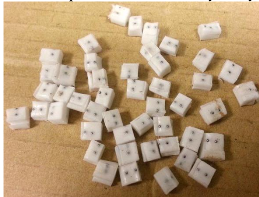
Figure 42: The beads embedded in plastic were successfully cut by hand into individual tags.
