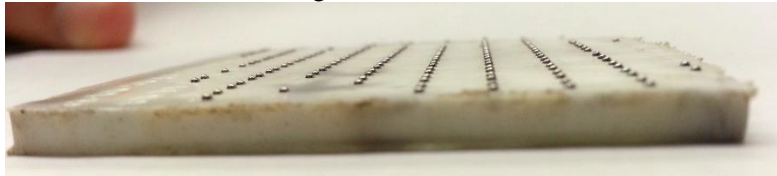
Figure 47: The sheet of microtags after being pressed between the bead plates. The beads do not implant far enough and tend to fall out.
