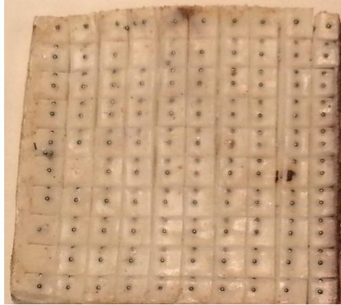
Figure 42: The beads embedded in plastic were successfully cut by hand into individual tags.
