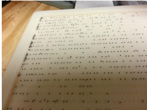
Figure 32: Tilted rapid prototype with excess beads at one side. These beads are difficult to remove.
