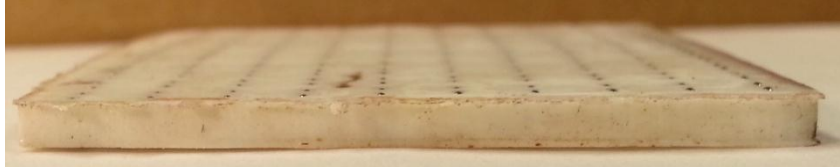
Figure 38: The flat plate press implanted the beads almost level with the surface.
