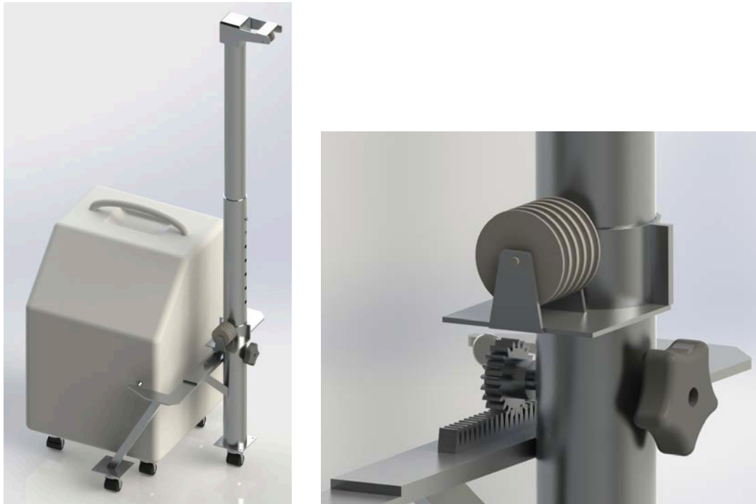
Figure 7: Alpha design on the left and close-up of clamping system and retraction device on the right.
