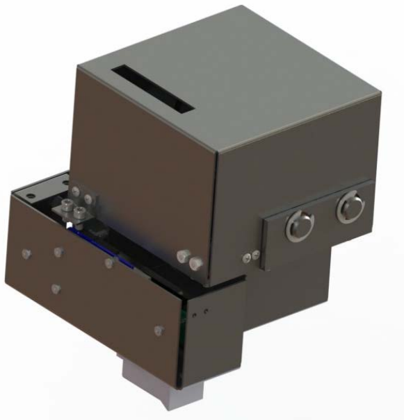
Figure 30: Both covers house the entire spool
