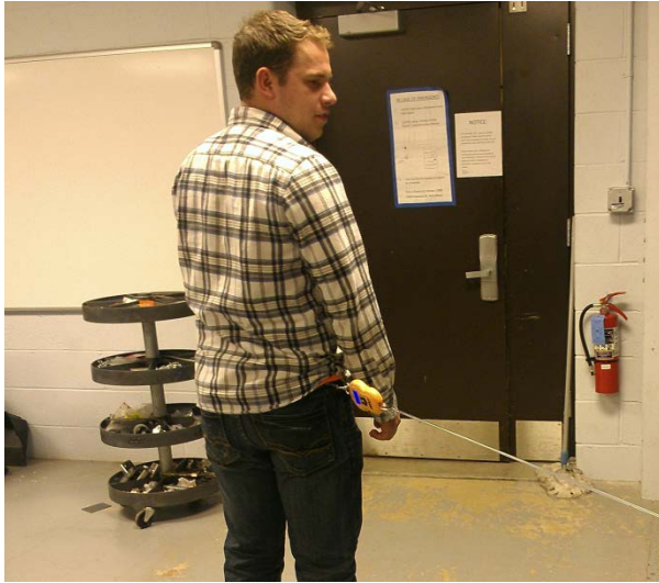
Figure 12: Set-up used for testing both minimum force felt on user and maximum force experienced by device.
