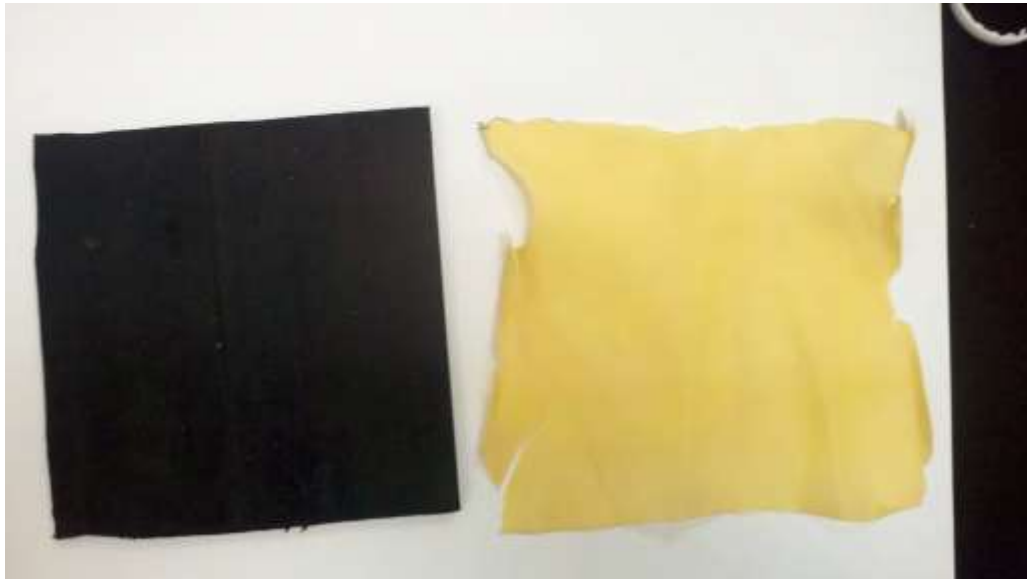
FIGURE 31: The undamaged control samples for NBR (left) and latex (right)
