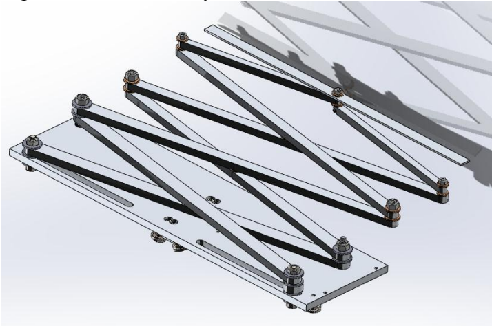
Figure 61: Extension by Means of a Scissor Mechanism
