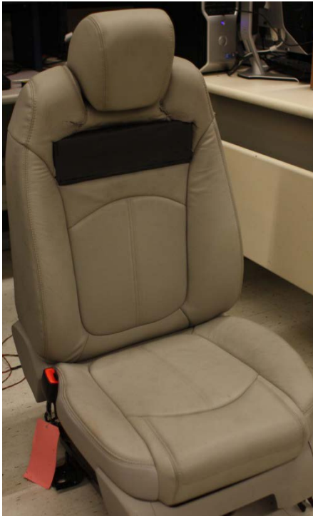
Xtendr Installed in Seat and In Fully Retracted Position
