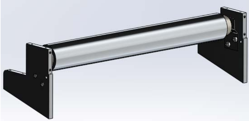
Figure 49: Spindle Mounted Between Brackets
