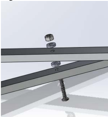
Figure 43: Pivot Points in Scissor Linkage
