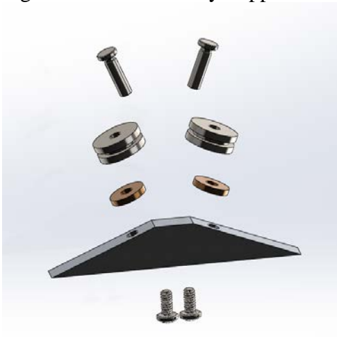
Figure 39: Lower Pulley Support
