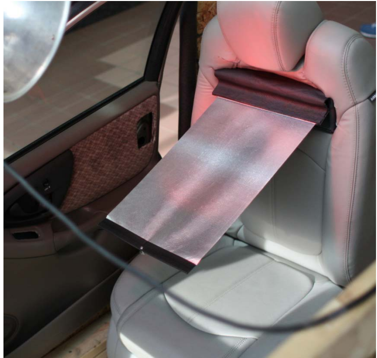
Xtendr at Design Expo in Fully Extended Position with Heat Lamp Demonstrating Radiation Blockage
