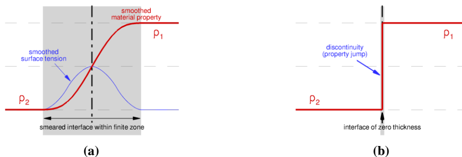
Figure 2. Interfacial dynamics modeling. (a) Fluid interface: continuous interface method with smeared interface within finite zone. (b) Solid interface: sharp interface method with the zero-thickness interface.
