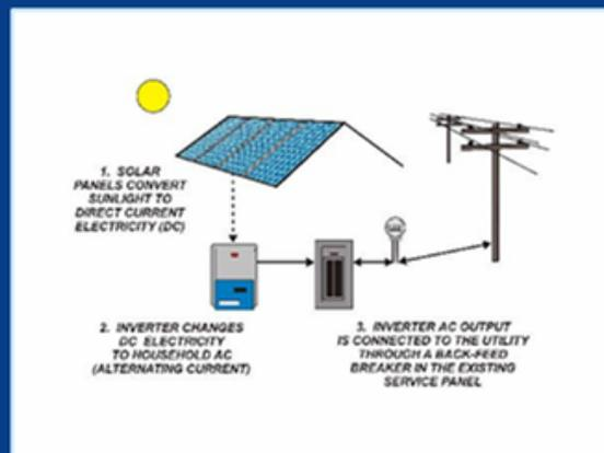
“The grid-tied power system allows a household to use as much energy as it needs, while selling the rest back to the power grid at the going electricity rate. In addition, if the system is underproducing due to weather or other conditions, the grid can serve as a backup without a disruption or power loss.
