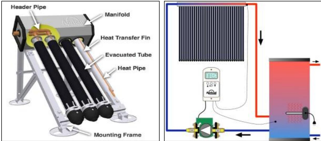
**Figure 17: Construction (left) and Operation (right) of an Apricus solar collector (Apricus, 2013).**
