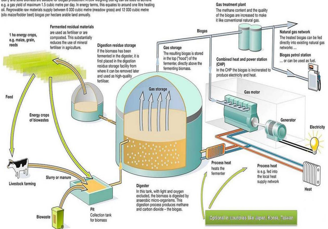
Figure 22: How a biogas digester operates (Biotec Asia Living Energy)
