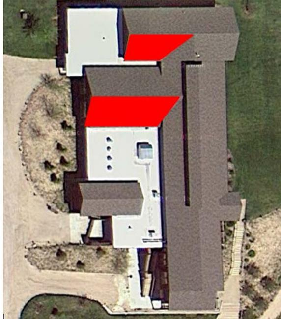
**Figure 25: Location of Recommended 19.76 kW Solar Photovoltaic System.** Area for solar modules indicated in red.
