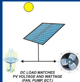
“The PV Direct Systems are the most simplistic solar installations available, and are used for much smaller purposes, such as powering a fan or a pump for a garden fountain, as shown here. The system is straight forward: the energy produced is used immediately for the purpose it’s been designed for. There is no conversion of energy types, and little to no power transmission required. And when the sun stops, the system stops, too.”
