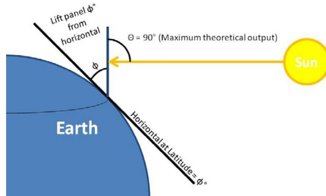
**Figure 9: Maximize panel output by tilting at angle equal to site latitude.**
