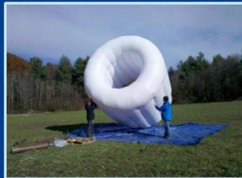
Altaeros Energies, Inc. offers one of several ideas to create an airborne version of the turbine, in this case using helium to lift the blades (located in the hollow center) as high as regular turbines, accessing the high wind velocities, while significantly reducing the costs of getting there.
