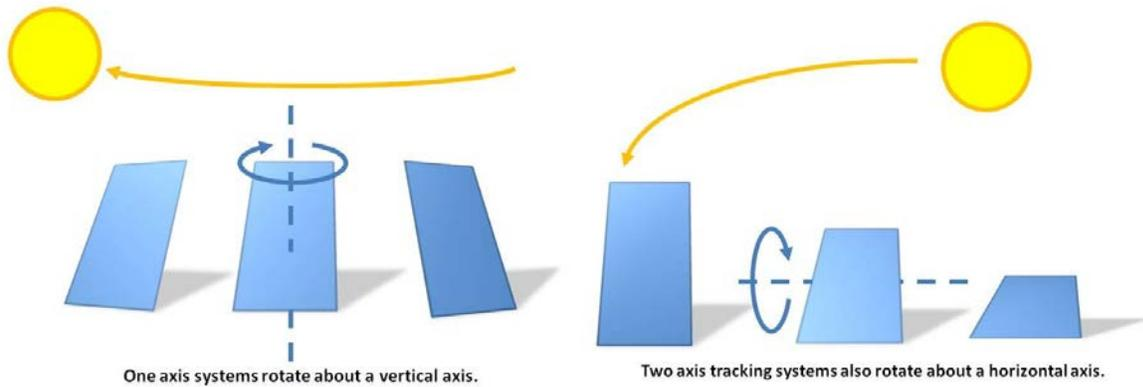
**Figure 8: One axis and two axis tracking systems rotate panels to face the sun.**
