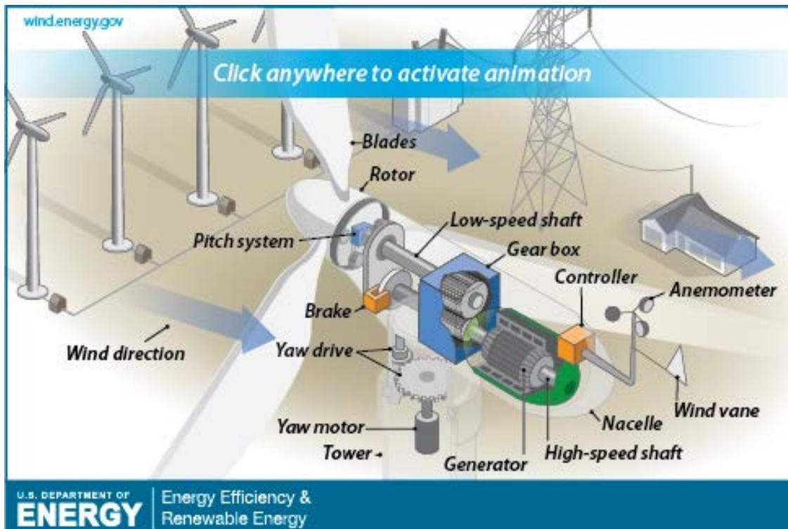
**Figure 19: The different parts of a wind turbine. (US DOE EERE)**
