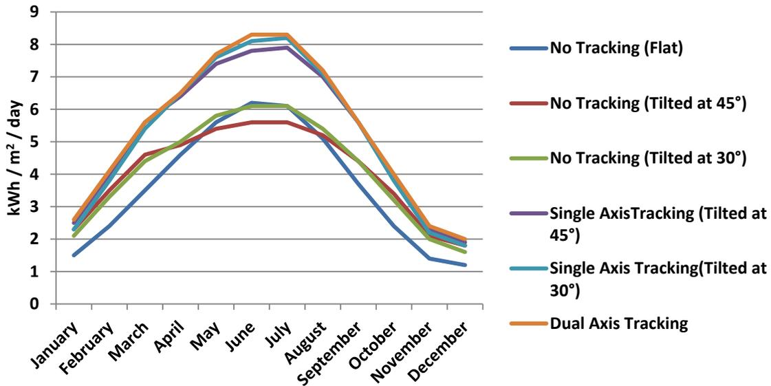
**Figure 10: 30 year average solar insolation for Traverse City, MI for various system configurations.** Adapted from (NREL, 1990)
