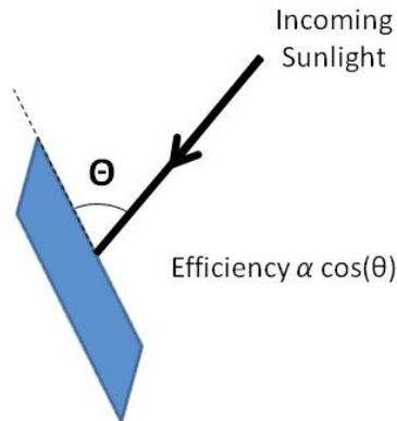
**Figure 7: Panel efficiency is proportional to the cosine of the angle of incidence.**
