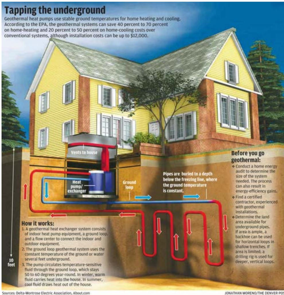
**Figure 23: Working of a geothermal heat pump for space heating and cooling (THB Energy Solutions)**
