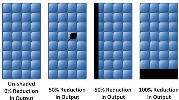
**Figure 11: Disproportionate single-panel reduction in power from partial shading.** Using microinverters or bypass diodes prevents this problem from adversely affecting the whole PV array. Adapted from (Wholesale Solar)
