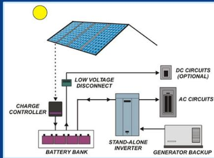
“A stand alone system has no connection to the grid and is instead connected to a battery operated system that stores extra energy directly on the premises, for use on the premises. The system stores enough energy to power an installation for several days and nights if the panels are disrupted or there is little no sun.
