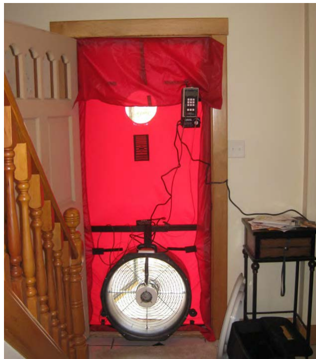
Figure 3. Blower door test to measure the rate of air infiltration (photo by Andrew Eilbert).
