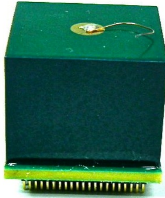
Figure 4.3: Picture of a 2 \text{ cm} \times 2 \text{ cm} \times 1.5 \text{ cm} CdZnTe detector. The planar cathode can be seen on top of the detector. The detector's pixels are connected to pins through a substrate on which the crystal is supported. The crystal is coated in order to remain protected from the light.
