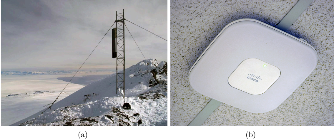
Figure 1.2: Common examples of radio repeaters: (a) High-level repeater [1]; (b) Low-level repeater (installed at the University of Michigan [2]).
