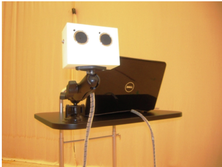
Figure 4.1. Picture of the measurement "Pixie" system consisting of a dual webcam assembly connected to a laptop.
