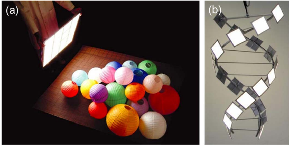
Figure 1-8: Examples of OLED lighting panels. (a) OLED lighting panels demonstrate a high color rendering index by illuminating colorful paper lanterns. (General Electric) (b) The form factor of OLEDs allows lighting to be integrated into aesthetically pleasing fixtures. (installation at Light + Building 2012)
