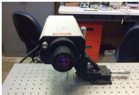
Figure 4.6: Schematic for measuring membrane displacement using laser vibrometer.
