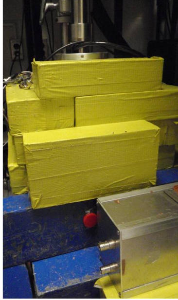
Figure 5.10: Picture of the setup used for measurements of ^{137}\text{Cs} gamma rays that are backscattered in the CdZnTe detector and absorbed in the HPGe detector.
