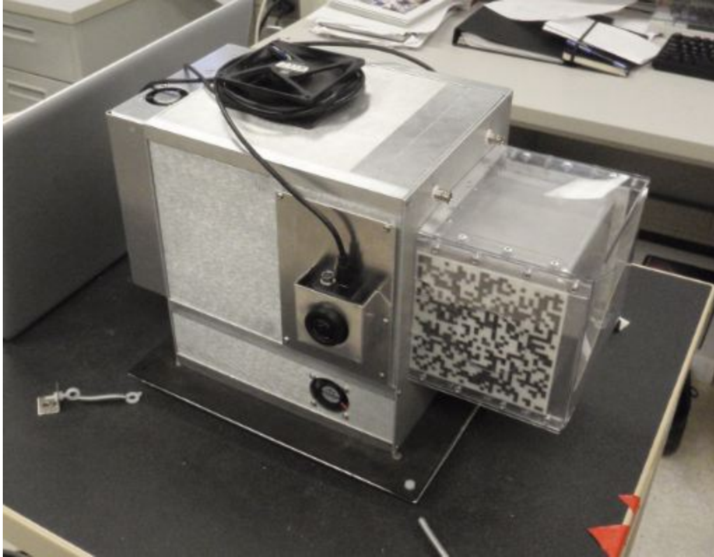
Figure 2.11: Picture of the second fully assembled CdZnTe array system complete with coded aperture masks and optical cameras.
