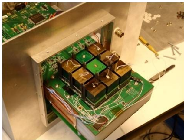
Figure 2.6: Picture of one of the populated MOCA boards placed in the first CdZnTe array system.
