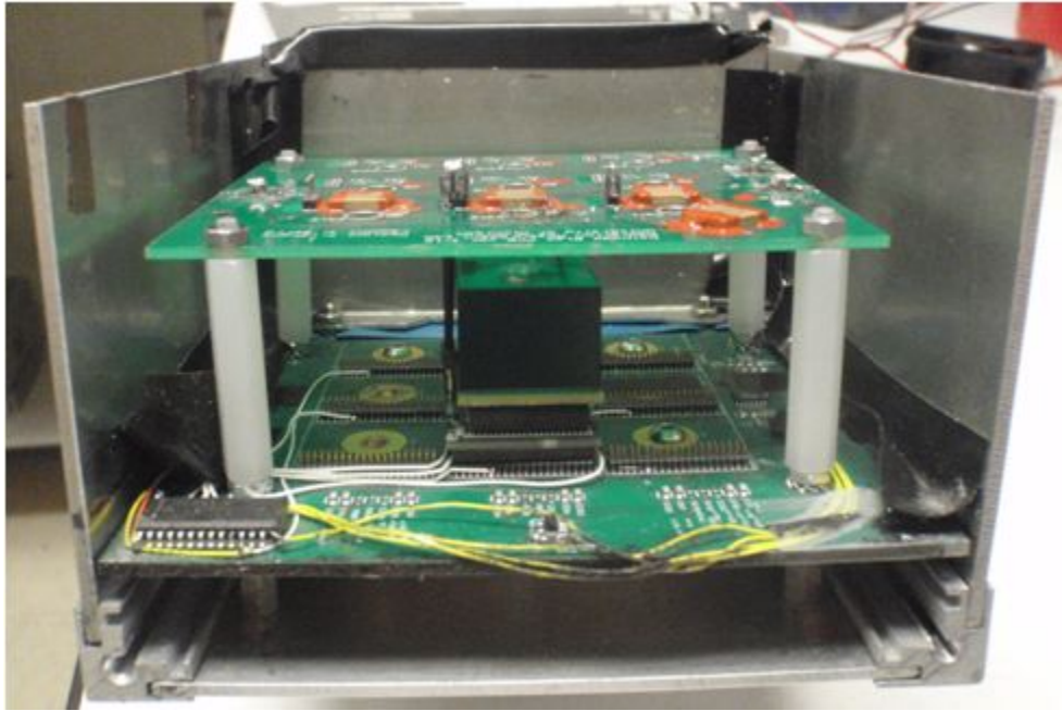
Figure 3.1: The setup of the test box for the CdZnTe detectors. Pictured is one of the 20 \times 20 \times 15 \text{ mm}^3 detectors mounted on a carrier board, which is plugged into an ASIC, which is then plugged into the motherboard. The motherboard is connected to a computer for data acquisition. Located above the detector is the high voltage distribution board, which is used to distribute the cathode and grid biases to the detector from external high voltage supplies.
