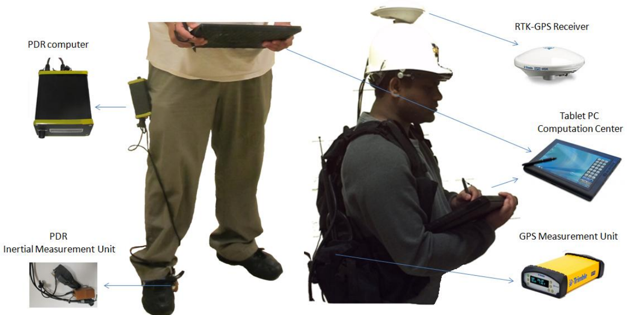
Figure A.1: RTK-GPS and PDR system hardware fitted on a mobile user
