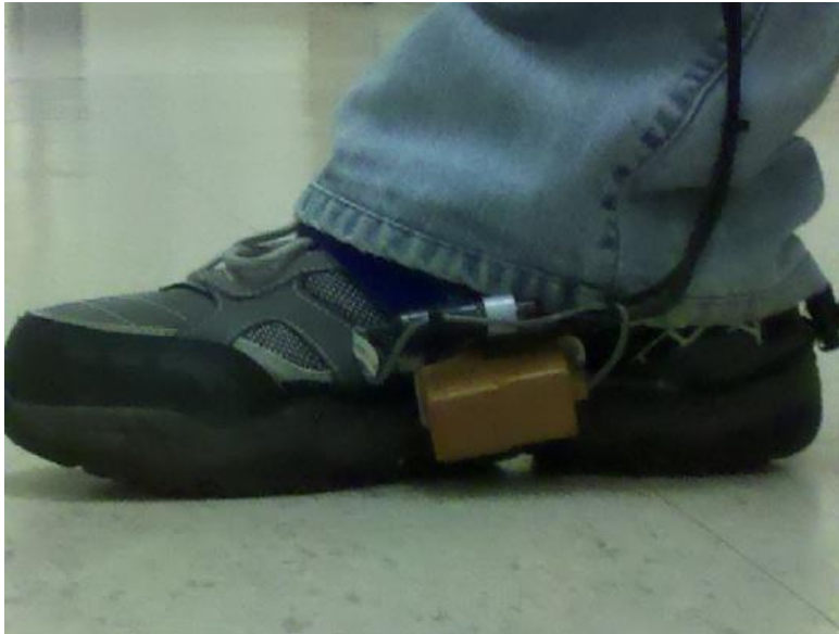
Figure 3.2: The small-sized nano IMU strapped onto a mobile user's foot
