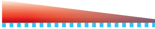
Figure 5.5: Schematic of surface adsorption evaporative cooling. The blue dashed line represents the silicon strips that are spaced evenly down the 1.5 m length of the guide. As the atomic beam travels, it is brought closer to the silicon surfaces. The hottest atoms adsorb onto the silicon, leaving the remaining atoms colder.
