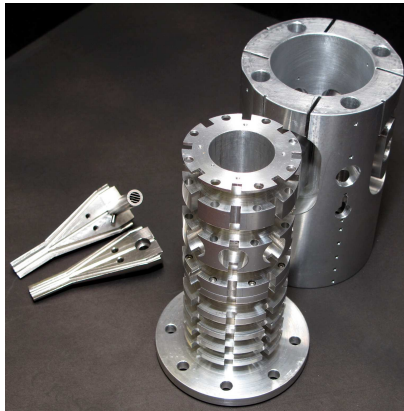
Figure 5.11: Jens Zorn took a few high-quality photographs of the pieces the Physics Instrument Shop machined for guide \beta . This shows the casing for the 2MOT, injection coil support, steel wire support, and mechanical shutter.
