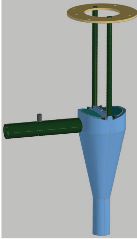
Figure 5.17: An Autocad depiction of the stainless steel wire holder and the stationary portion of the shutter.
