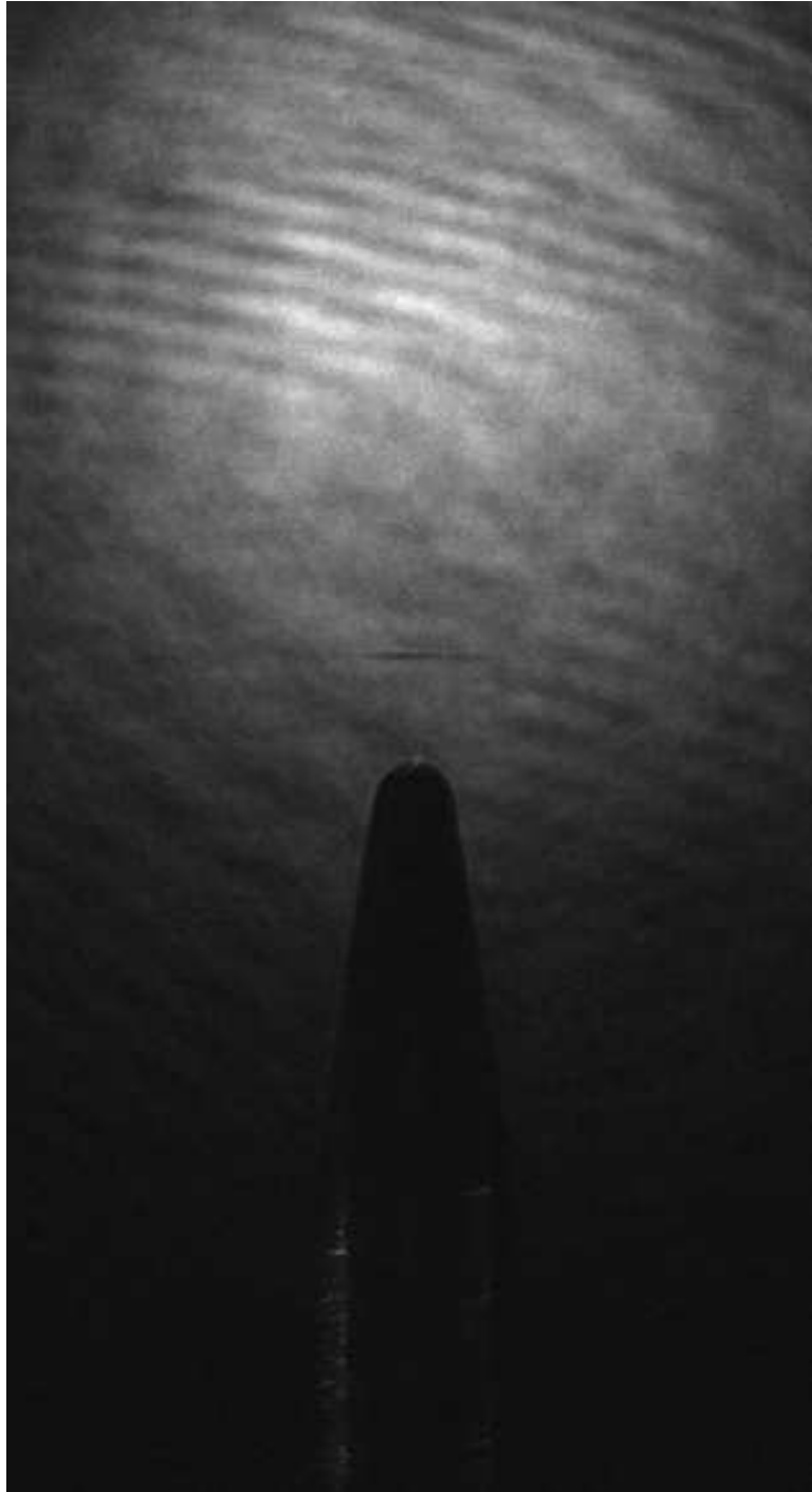
Shadow image of the TIP 1 , and above it an optical dipole trap.
