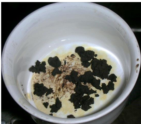
Figure 3.3. Chlorella hydrochar obtained from reaction at 250° C for 30 min
