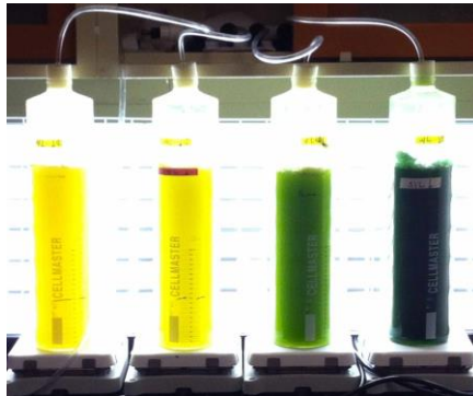
Figure 7.4. Bubble column reactors (BCRs) in a nutrient replete state (green) and nutrient-deprived state (yellow).
