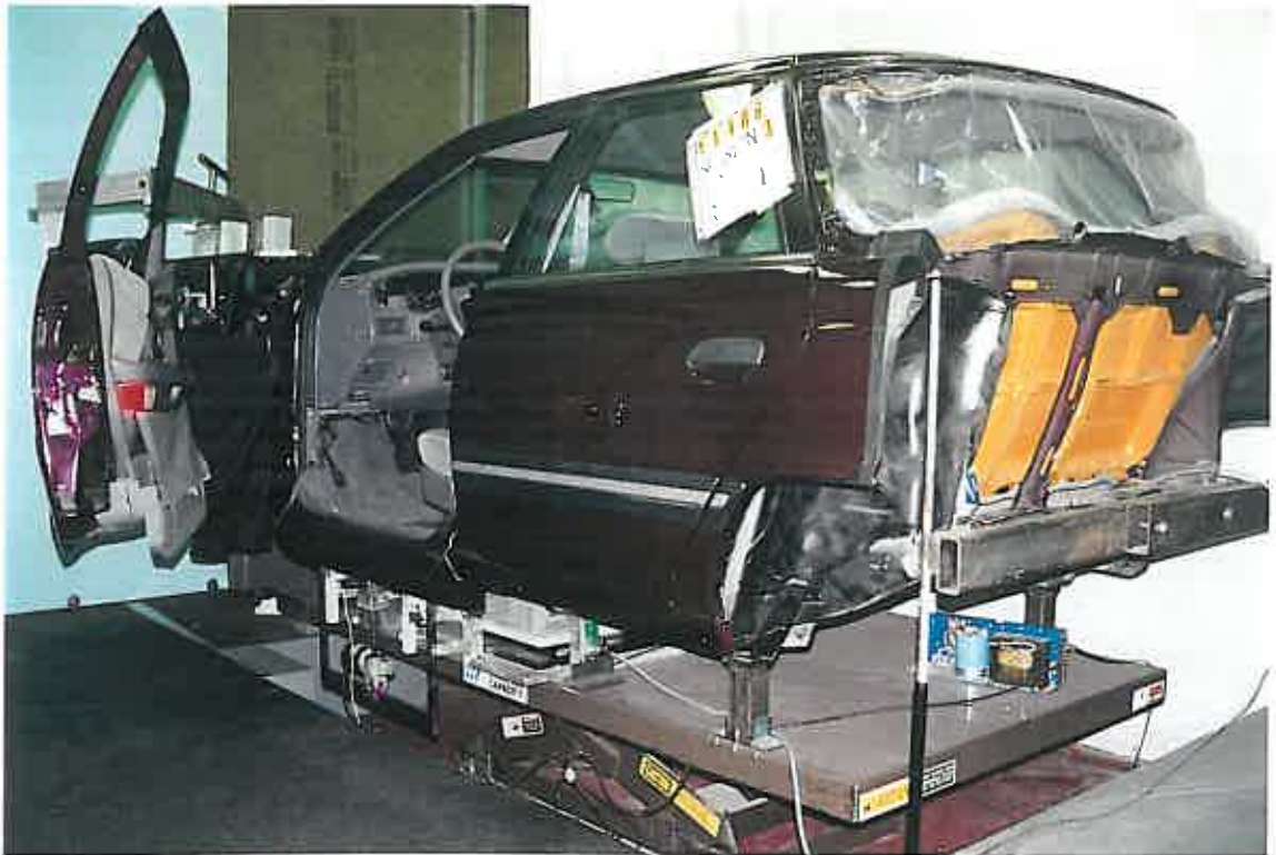
Figure H.2 Overview of ingress/egress test buck with high seat-to-ground distance.
