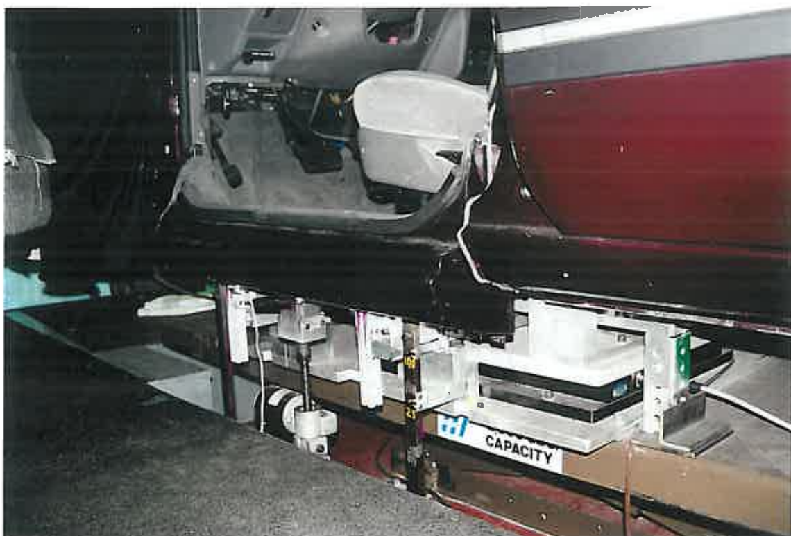
Figure H.8 Rocker height adjustment mechanism with rocker in high (100 above AHP) position.
