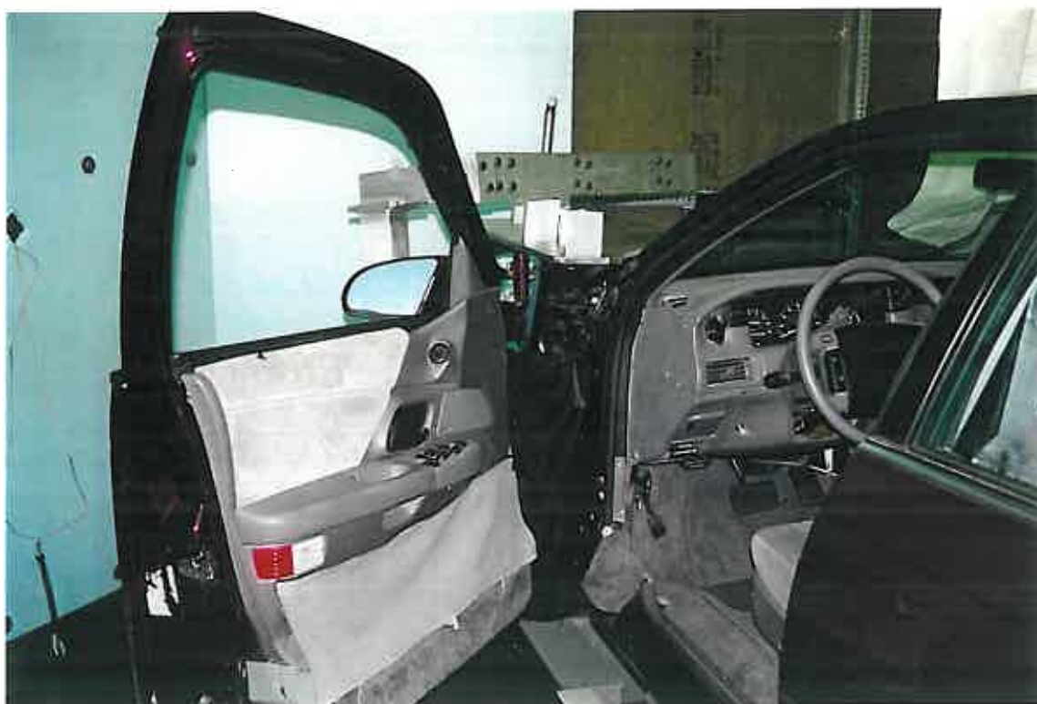
Figure H.5 Door of ingress/egress test buck opened using 4-bar (a) linkage condition.
