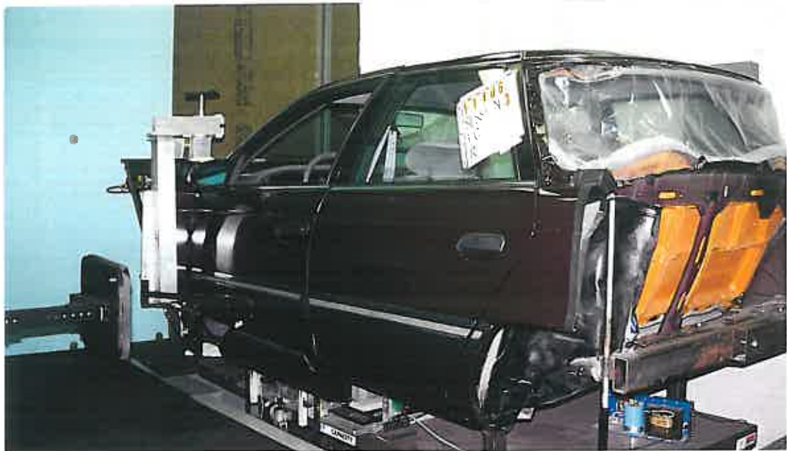
Figure 2a. Photograph of the laboratory ingress/egress buck.
