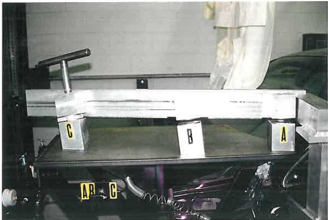
Figure 4b. Three-pivot mechanism attached to ingress/egress test buck used to simulate production and four-bar mechanism door hinge scenarios (See Appendix H for additional photos).
