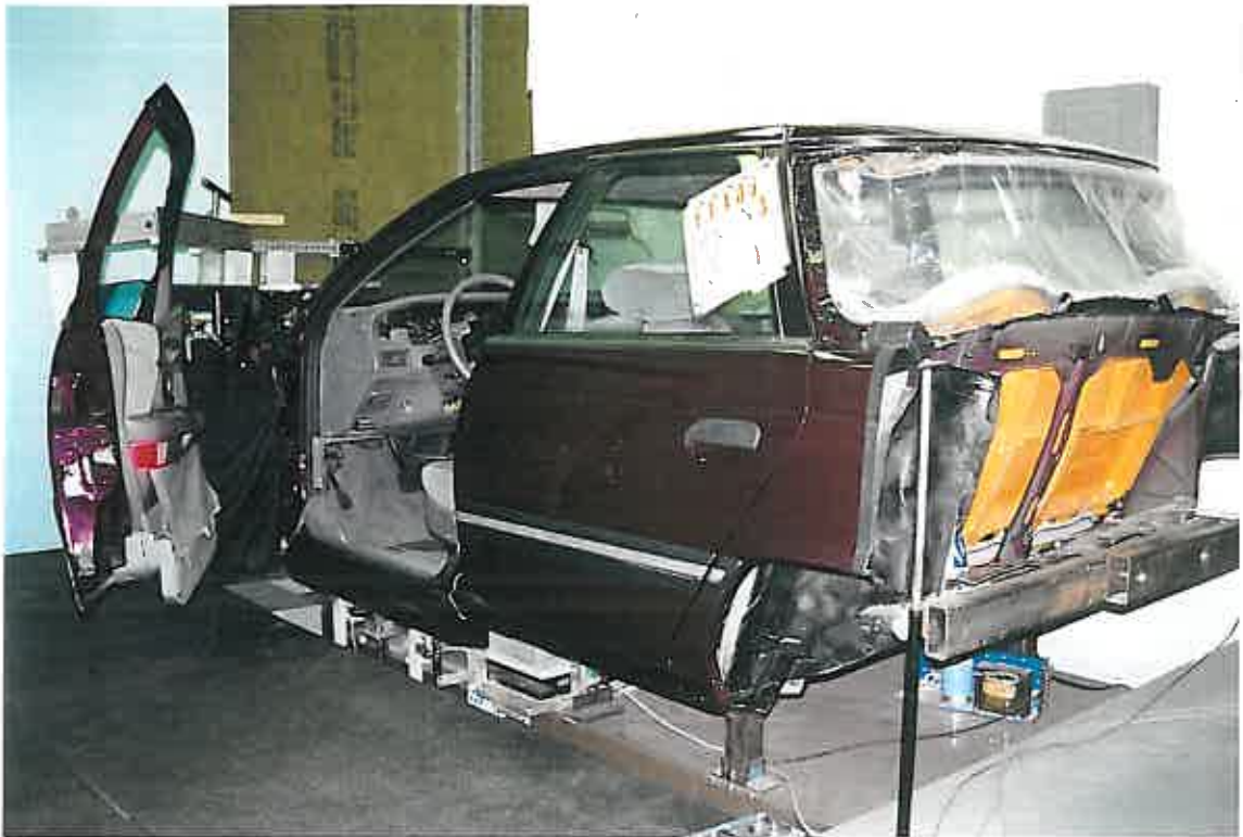
Figure H.1 Overview of ingress/egress test buck with low seat-to-ground distance.
