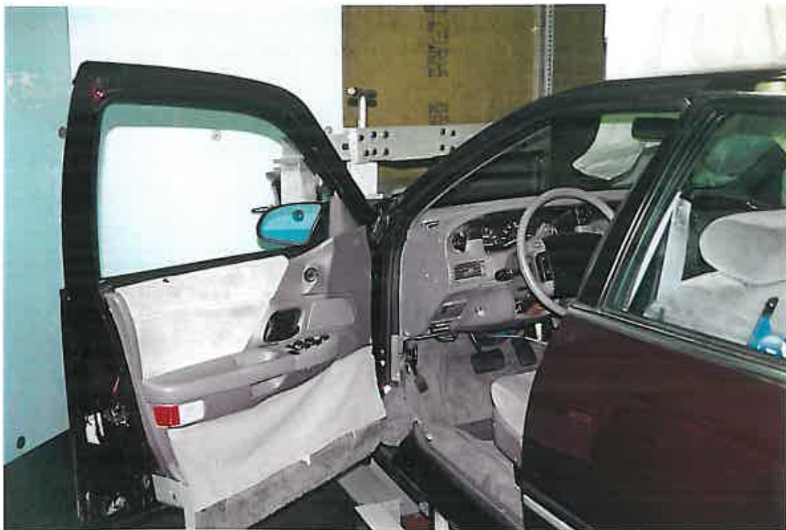
Figure H.4 Door of ingress/egress test buck opened using production pivot hinge position.
