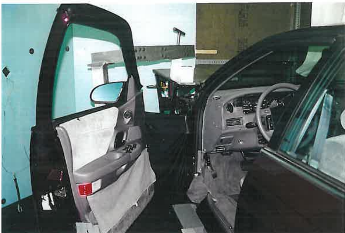
Figure H.6 Door of ingress/egress test buck opened using 4-bar (b) linkage condition.
