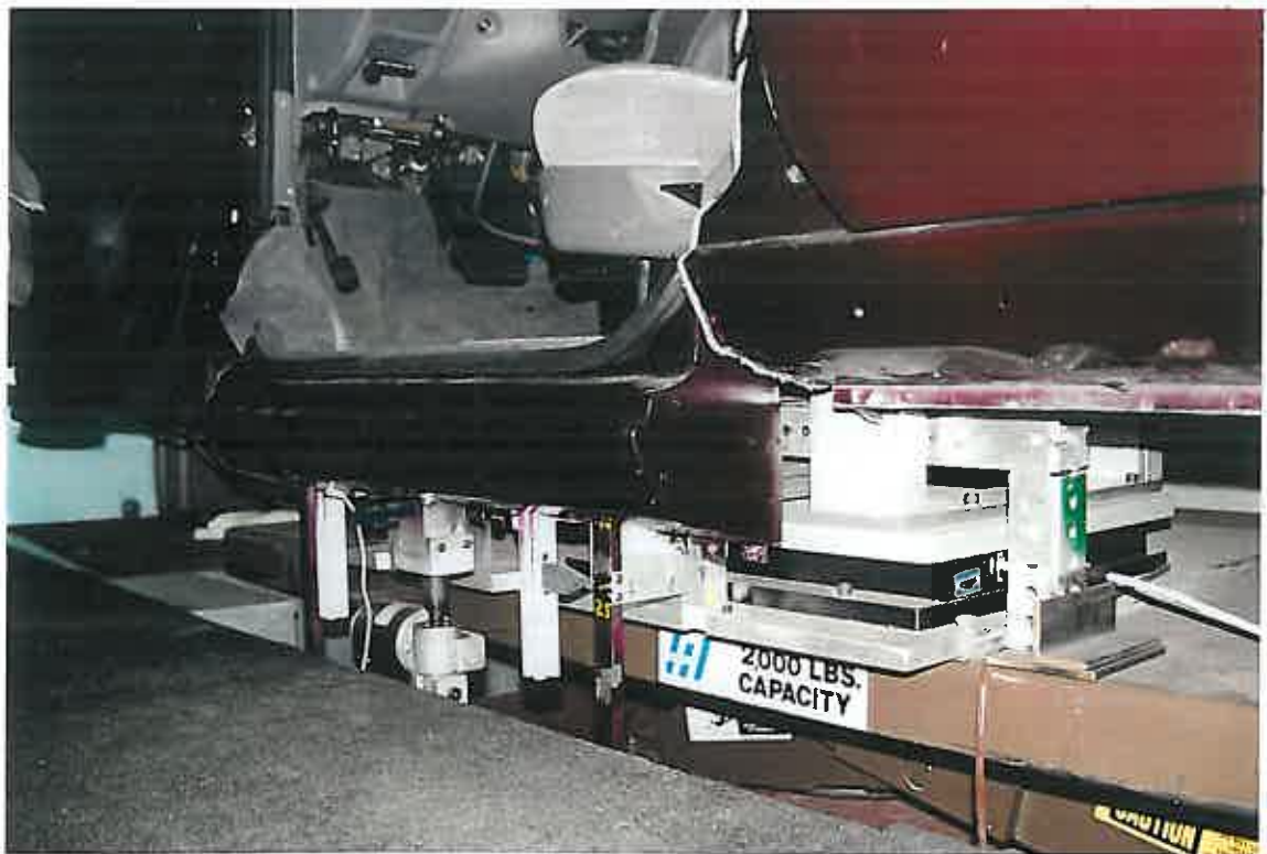
Figure H.7 Rocker height adjustment mechanism with rocker in low (25 mm above AHP) position.
