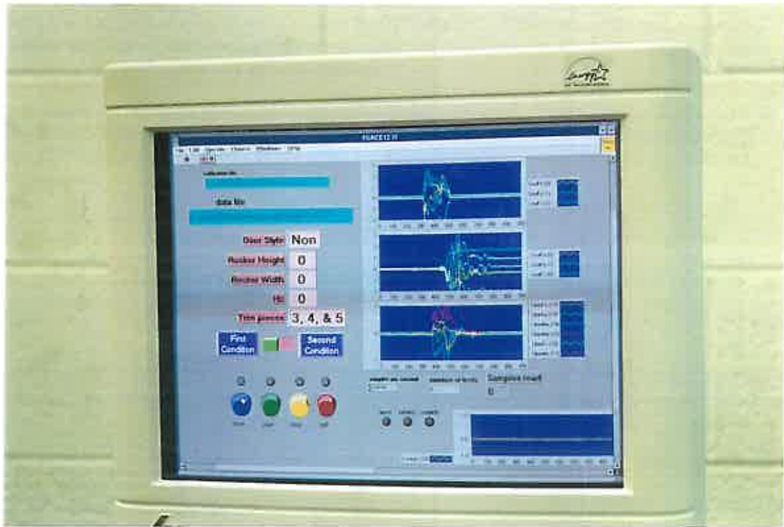
Figure 6. Display of force signals on computer screen using LabView.
