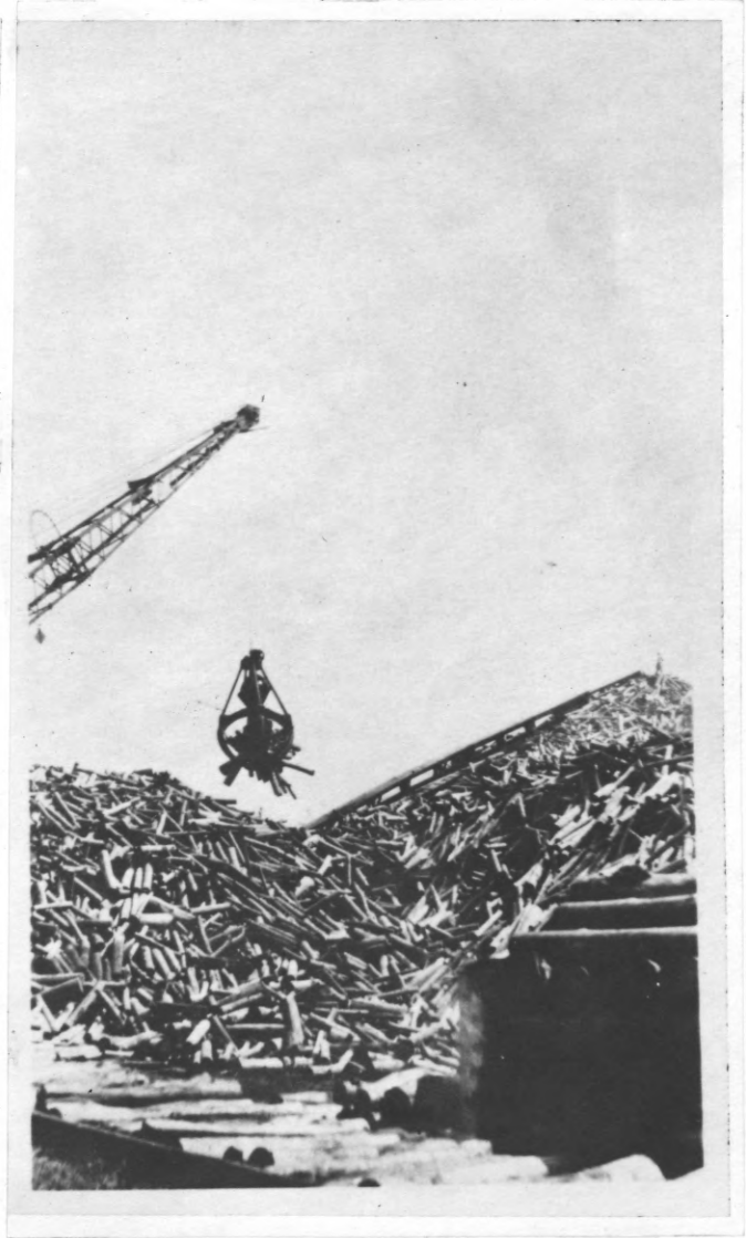
Figs. 28 and 29. An "orange-peel" grapple for handling pulpwood in conical piles.
