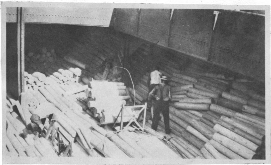
Fig. 24. Method of unloading. A sling is laid in the cord frame on which the sticks are piled ready for hoisting by a derrick.
