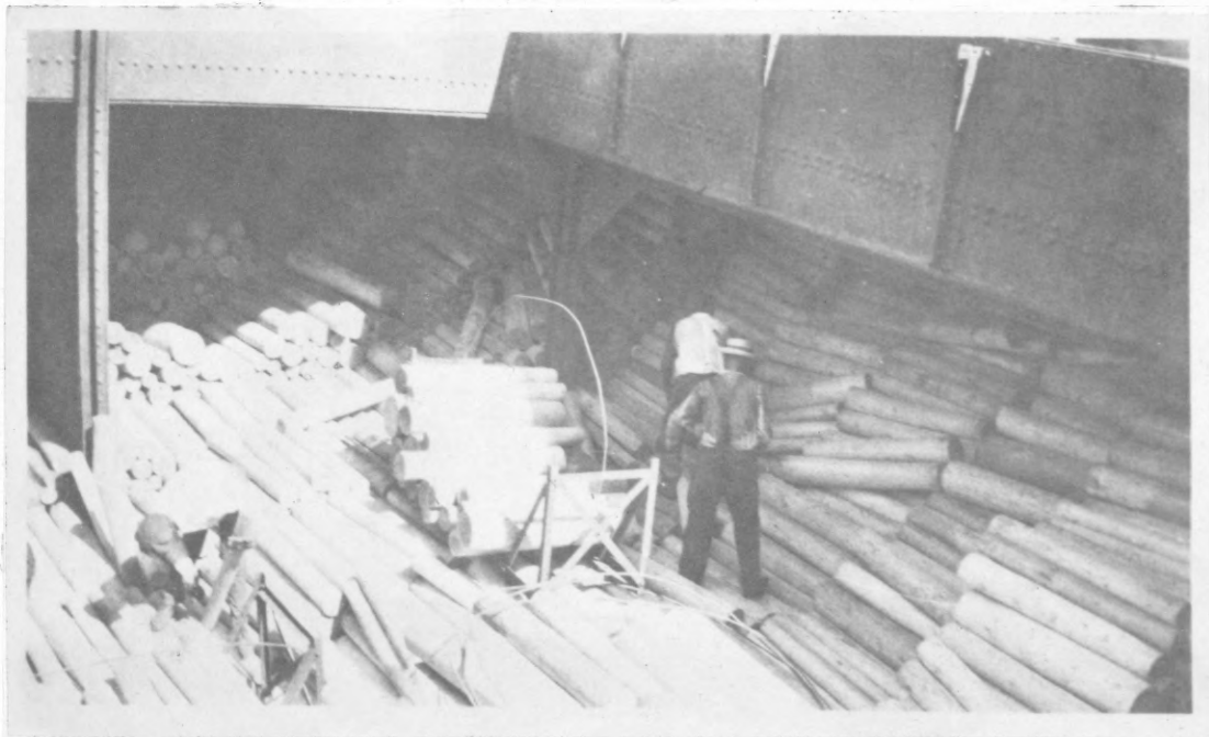
(Fig. 20) Workers in hold of ship making up bundles of pulpwood to be lifted from hold by means of cranes.
