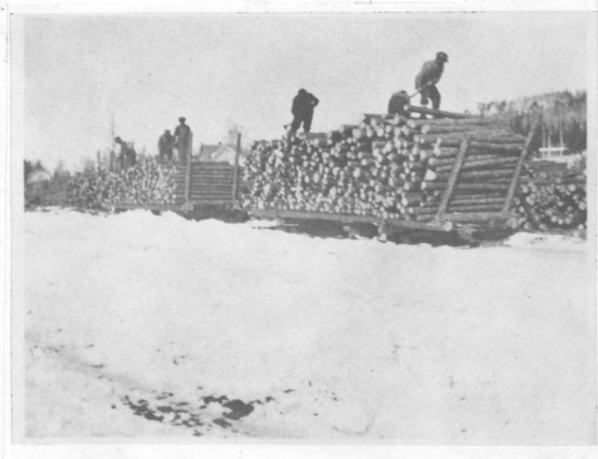
(Fig. 4) Unloading pulpwood from sleight to river. (Note use of "pickaroons" in handling wood.)
