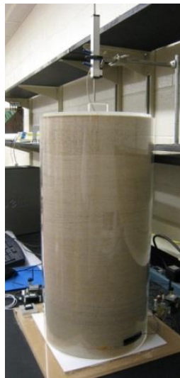
Figure 4.58. Cylinder test set-up for detecting time-dependent behavior of sand (cylinder diameter: 30 cm).
